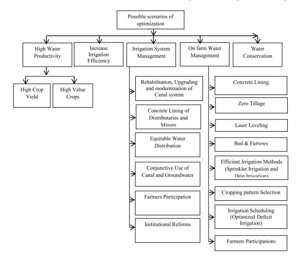
Fig. 5. Schematic Diagram of Optimization of irrigation water management at canal command level.
