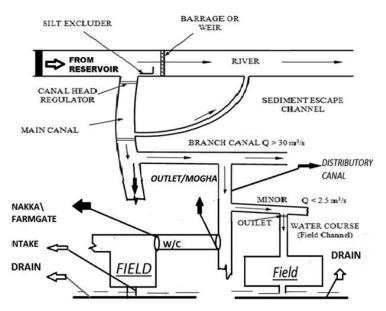
Fig. 4. Schematic Diagram of Typical Irrigation system of Pakistan
