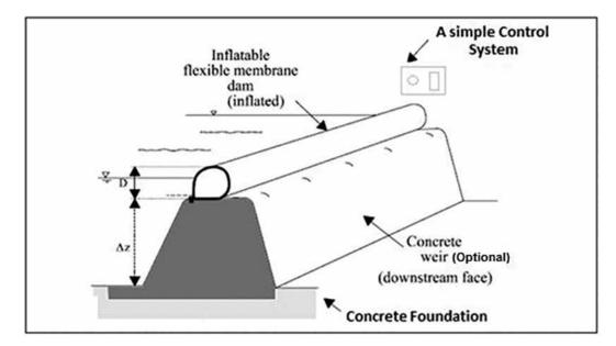
Fig. 2. Schematic view of inflatable Rubber Dam.
