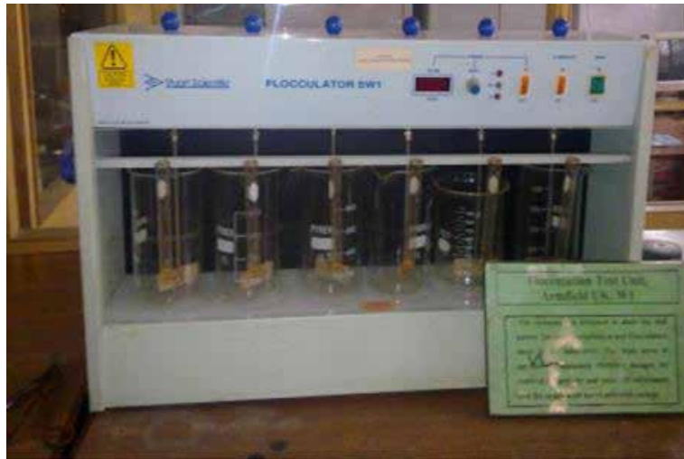
Fig. 2. Experimental setup consisting of coagulation and flocculation unit.
