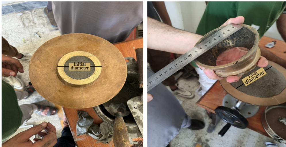
Fig. 4. Setup for measuring mortar flow using a flow table.
