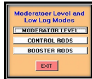
Fig. 7. GUI for reactivity transient selection of moderator level mode in low power operation.
