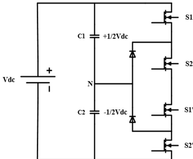
Fig. 9. One leg of typical NPC inverter
