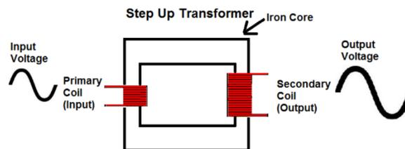
Fig. 13. Working of step-up transformer
