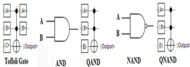
**Fig. 1.** By fixing the Toffoli gate’s third qubit to  $|0\rangle$  or  $|1\rangle$ , the classical AND and NAND gates are transformed into Quantum AND and Quantum NAND gates respectively. Where inputs ( $|A\rangle$ ,  $|B\rangle$ ) and  $|C\rangle$  are named as Qubits (quantum states) with A and B being classical bits (0 or 1) [28-30].
