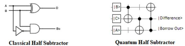
**Fig. 6.** Classical Half Subtractor is transformed into quantum Half Subtractor with two CNOT gates and one Toffoli gate acting on different qubits. Where, inputs ( $|A\rangle$ ,  $|B\rangle$ ) and  $|C\rangle$  are named as Qubits (quantum states), A and B are classical bits (0 or 1), D (Difference) and B (borrowed) are classical outputs (0 or 1) [28-30].
