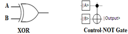
Fig. 3. CNOT gate of quantum computing is equivalent of Classical XOR gate. Where, inputs ( |A\rangle , |B\rangle ) and |C\rangle are named as Qubits (quantum states) and A and B are classical bits (0 or 1) [28-30].
