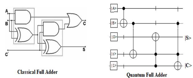
**Fig. 5.** Classical full adder is transformed into quantum full adder with CNOT gate and three Toffoli gates acting on different qubits. Where, inputs ( $|A\rangle$ ,  $|B\rangle$ ) and  $|C\rangle$  are named as Qubits (quantum states) and A, B, S (Sum), and C (Carry) being classical bits (0 or 1) [28-30].
