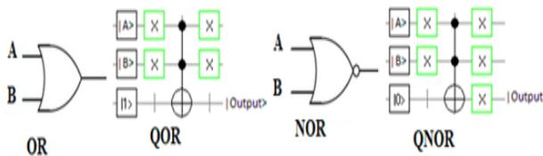
**Fig. 2.** By fixing third qubit of Toffoli gate to be  $|1\rangle$  or  $|0\rangle$ , the classical OR and NOR gates are transformed into QOR and QNOR gates respectively. Where, inputs ( $|A\rangle$ ,  $|B\rangle$ ) and  $|C\rangle$  are named as Qubits (quantum states) and A and B are classical bits (0 or 1) [28-30].
