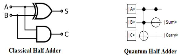
**Fig. 4.** Classical half adder is transformed into quantum half adder by applying Toffoli gate on the three qubits followed by CNOT gate applied to the first two qubits. Where, inputs ( $|A\rangle$ ,  $|B\rangle$ ) and  $|C\rangle$  are named as Qubits (quantum states), and A, B, S (Sum), and C (Carry) are classical bits (0 or 1) [28-30].
