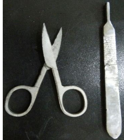
Fig. 6. Surgical tools prepared via powder metallurgy temperature calculated by Archimedes principle
