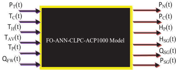
Fig. 2. FO-ANN-CLPC input-output MIMO configuration model of ACP1000.
