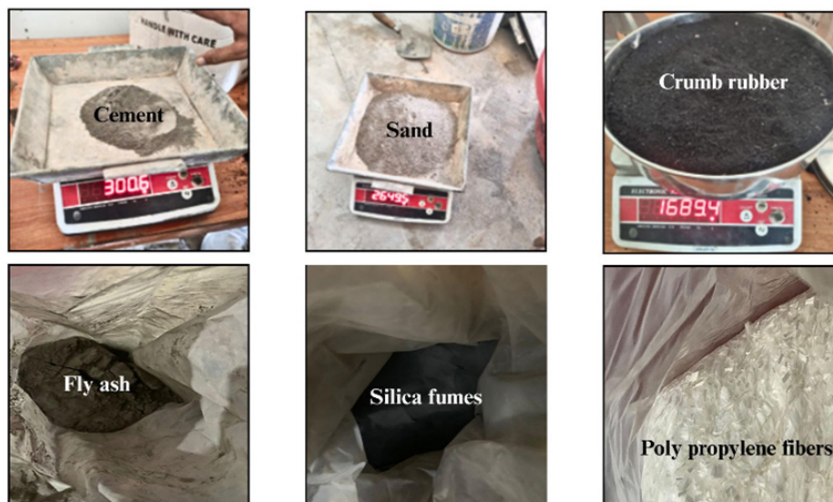
Fig. 1. Raw materials used for producing control and rubberized cementitious mortars.
