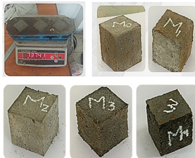
Fig. 2. Mortar casting process from three-gang mold to hardened cube specimens.
