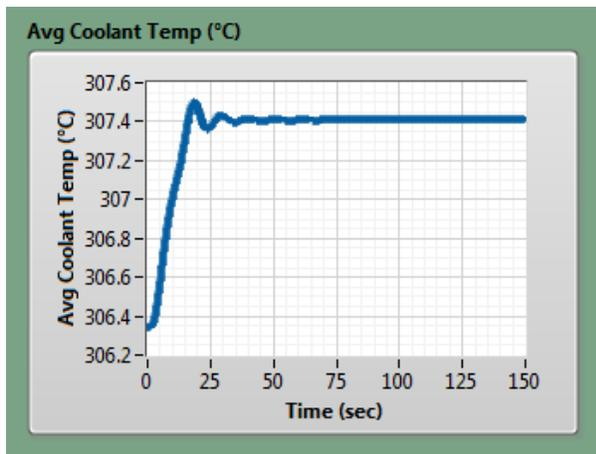
Fig. 7. Optimization of average coolant with linear control rod reactivity model in LabVIEW
