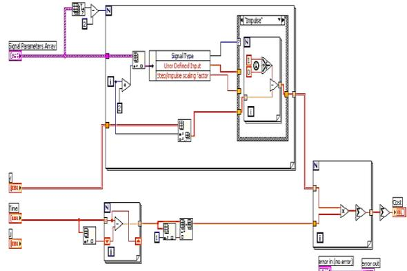
Fig. 9. Design of cost function for nonlinear SQP optimization VI in LabVIEW
