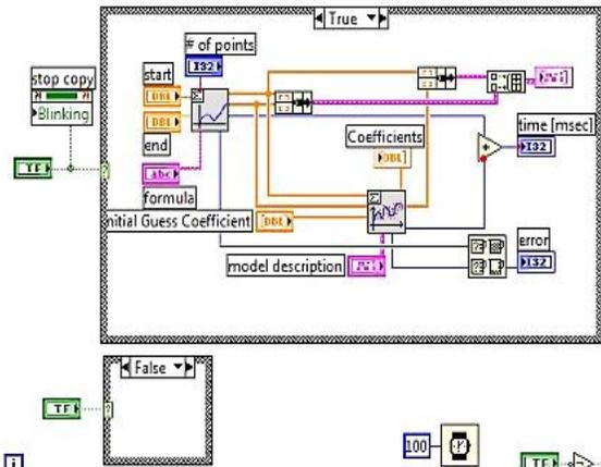
Fig. 13. Calibration of neutronics and thermal hydraulics system model in LabVIEW
