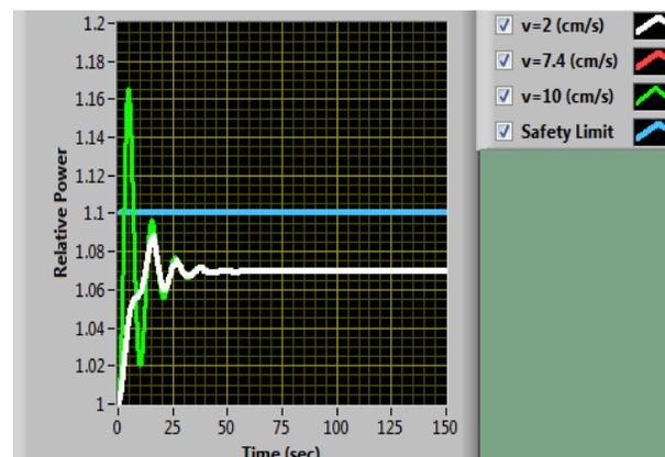
Fig. 6. Optimization of relative reactor power with linear control rod reactivity model in LabVIEW
