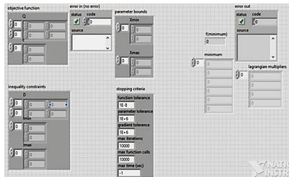
Fig. 10. Design of front panel for nonlinear SQP optimization VI in LabVIEW
