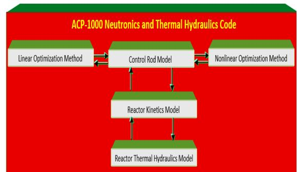
Fig. 1. Framework of ACP1000 neutronics and thermal hydraulics modeling.
