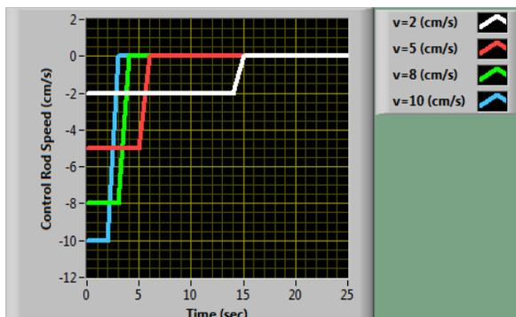
Fig. 4. Optimization of control rod speed with linear control rod reactivity model in LabVIEW
