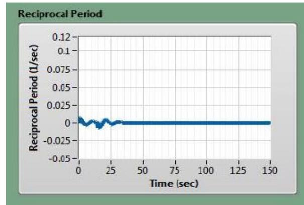
Fig. 5. Optimization of reciprocal reactor period at optimal control rod speed with linear control rod reactivity model in LabVIEW
