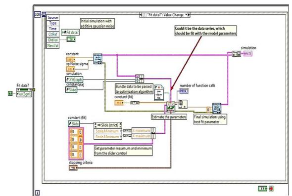
Fig. 11. Computation of neutronics and thermal hydraulics system model parameters in LabVIEW
