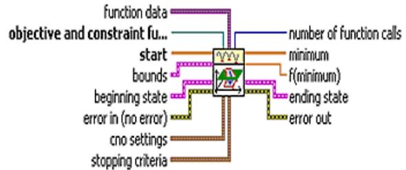
Fig. 8. Design of nonlinear SQP optimization VI in LabVIEW
