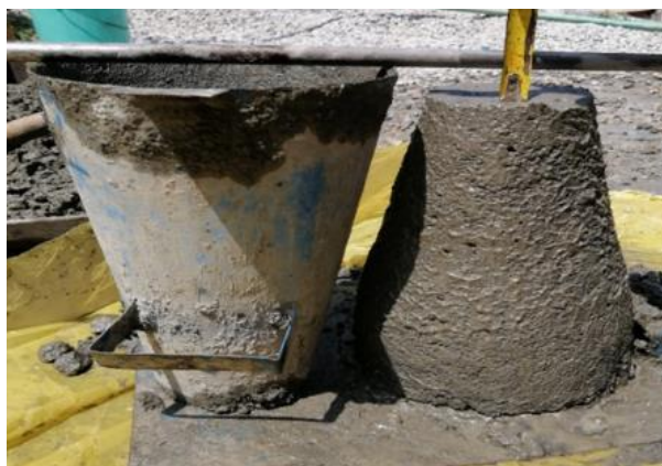
Fig. 3. True slump in rubberized concrete containing 10% crumb rubber.
