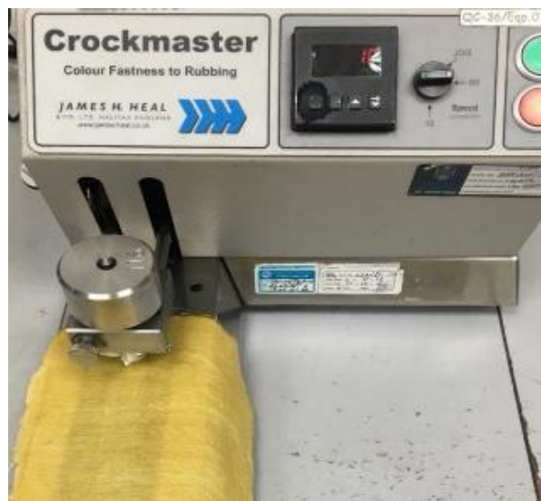
Fig.2. Colorfastness of samples through Crock meter
