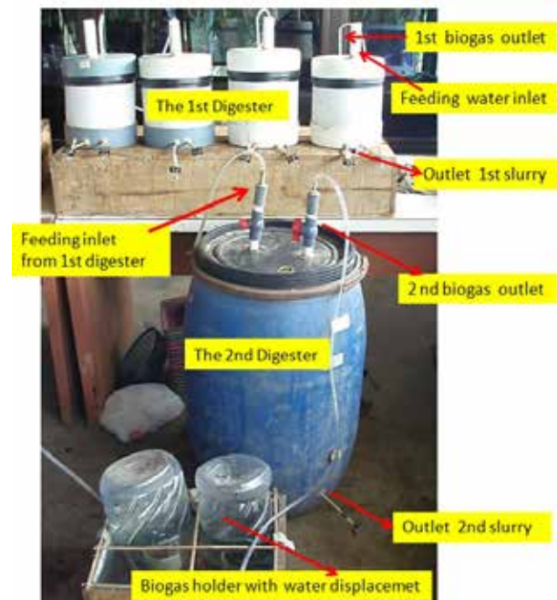
Fig. 1. The first and second digester.
