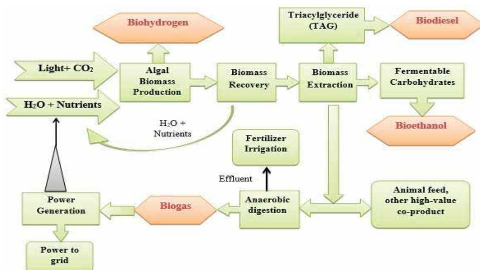
**Fig. 3.** A conceptual model for integrated microalgal biomass and biofuel production [5].
