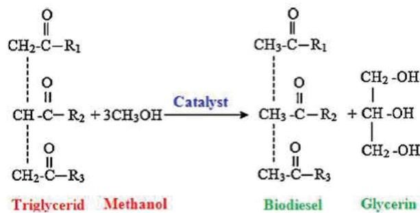
Fig. 4. The transesterification process of conversion of triglyceride into biodiesel [57].
