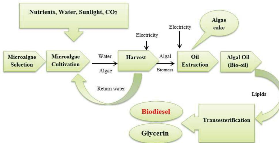
Fig. 5. Schematic representation of the various stages of manufacture of microalgal biodiesel [30]
