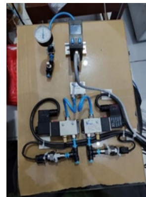
Fig. 7. The oxygen flow installation.
